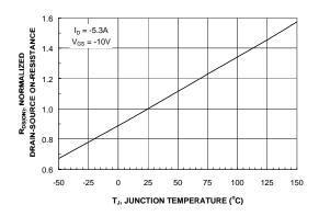
Figure 3. On-Resistance Variation with Temperature.
