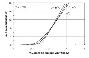
Figure 5. Transfer Characteristics.
