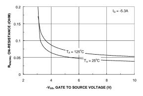
Figure 4. On-Resistance Variation with Gate-to-Source Voltage.
