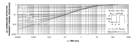
Figure 11. Transient Thermal Response Curve.
