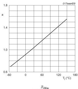
$$a = \frac{R_{DSon}}{R_{DSon(25^{\circ}C)}}$$
