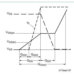
Fig 15. Gate charge waveform definitions
