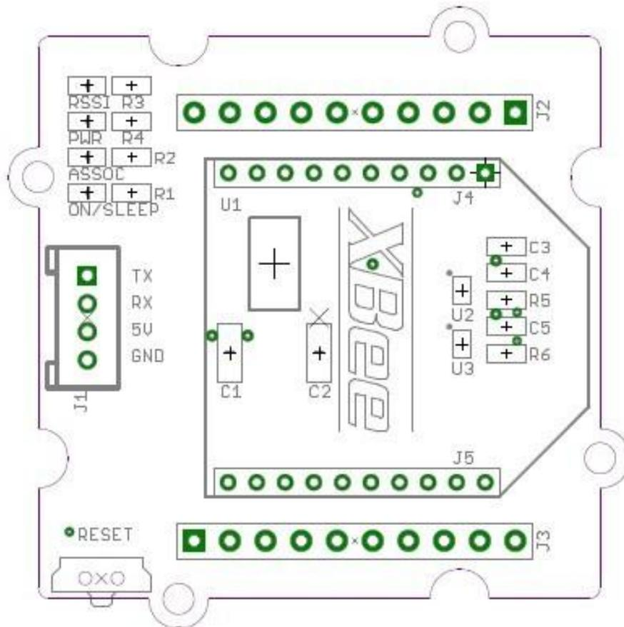
**J1:** Grove Interface, used for connecting to UART Interface of Arduino/Seeeduno.
