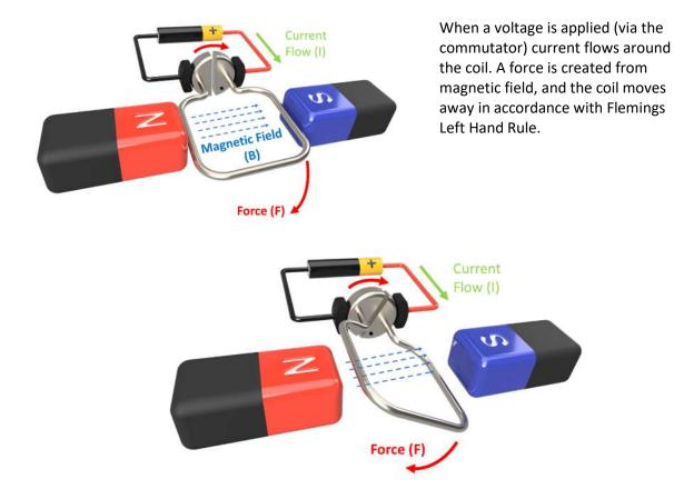
As the coil rotates towards the opposite side the force would change direction, and the motor would not spin. To prevent this the commutator switches the current to flow in the opposite direction through the coil, which then continues to rotate.
