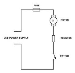
The circuit diagram for the USB Fan is shown above. It is a very simple circuit. The 5V that powers the circuit is supplied from the USB connector.
