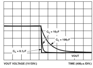
FIGURE 9. FAST TURN-OFF vs CLOAD
