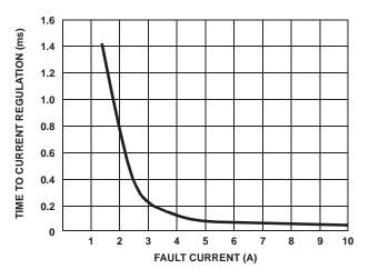
FIGURE 7. CR SETTLING TIME vs FAULT CURRENT
