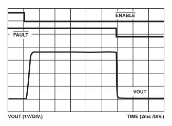
FIGURE 10. ISL6436L TURN-ON INTO 1.5A OCS
