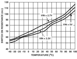
FIGURE 2. SWITCH ON RESISTANCE AT 0.7A
