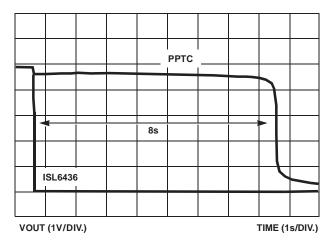
FIGURE 15. ISL6436 vs PPTC WITH EXTENDED 1.5A LOAD
