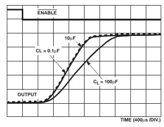
FIGURE 3. VOUT SOFT START vs C<sub>LOAD</sub>, RI =10 $\Omega$
