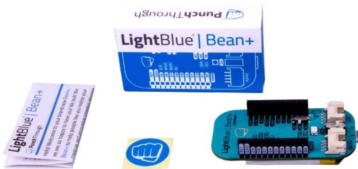
It is an Arduino-compatible board that you program wirelessly using Bluetooth Low Energy. With Bean+, you can program wirelessly from any of your devices. Bean+ also comes with a built-in accelerometer, temperature sensor and RGB LED.
