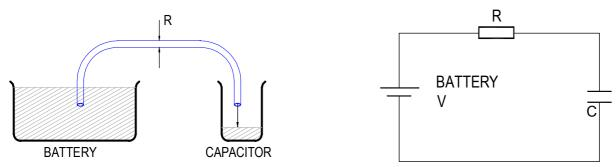
When a capacitor is connected to an item such as a battery, charge will flow from the battery into it. Therefore the capacitor will begin to fill up. The flow of water in the picture above left is the equivalent of how the electrical charge will flow in the circuit shown on the right.
