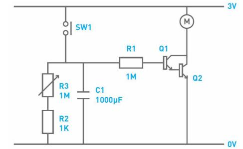
When the switch (SW1) is pressed the capacitor (C1) charges. When the switch is released the capacitor (C1) slowly discharges through the resistors (R2 & R3). R2 is just present to make sure that the batteries aren't shorted if the switch is pressed and the variable resistor R3 is set to zero.
