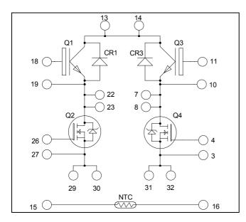
Top switches: Trench + Field Stop IGBT3
