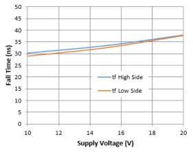
Figure 10. Fall Time vs. Supply Voltage
