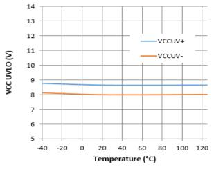
Figure 26. VCC UVLO vs. Temperature
