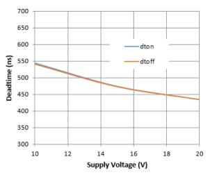
Figure 24. Deadtime vs. Supply Voltage
