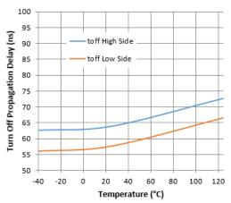
Figure 7. Turn-off Propagation Delay vs. Temperature
