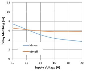
Figure 14. Delay Matching vs. Supply Voltage
