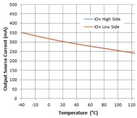
Figure 17. Output Source Current vs. Temperature
