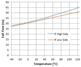
Figure 11. Fall Time vs. Temperature
