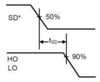
Figure 2. Shutdown Waveform Definition
