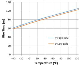
Figure 9. Rise Time vs. Temperature
