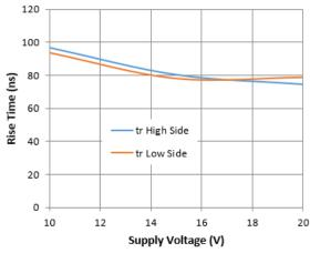
Figure 8. Rise Time vs. Supply Voltage
