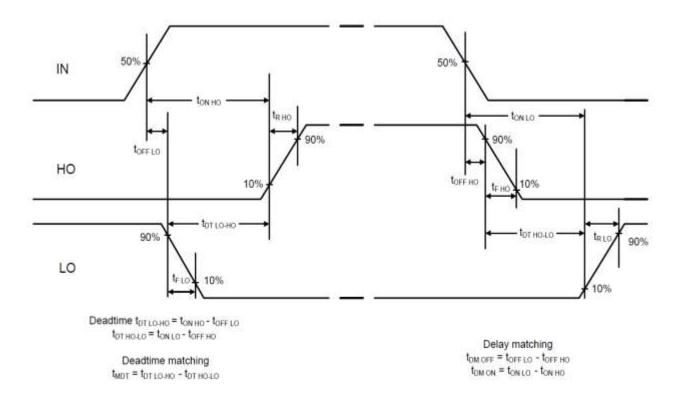
Figure 3. Switching Time Waveform Definitions
