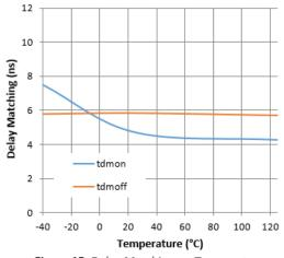
Figure 15. Delay Matching vs. Temperature
