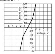
9. Off state leakage current Measured portion: between terminals 7 and 8
