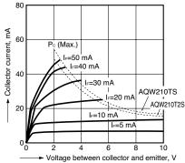
4-2. Collector current vs. voltage between collector and emitter characteristics (Ic-VcE) Measured portion: between terminals 3 and 4 (AQW210TS), 3 and 4, 5 and 6 (AQW210T2S) Ambient temperature:  $25^{\circ}$ C  $77^{\circ}$ F
