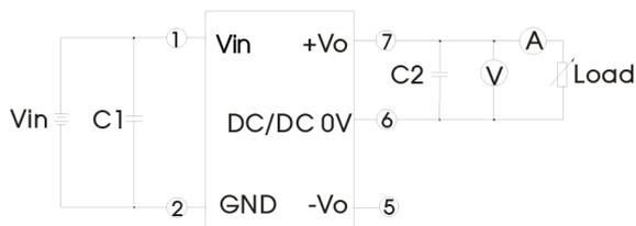
Note: C1,C2,C3: 100uF/35V (Low internal resistance capacitance)
