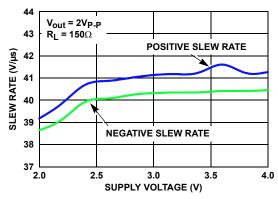
FIGURE 19. SLEW RATE vs SUPPLY VOLTAGE
