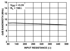
FIGURE 18. -3dB BANDWIDTH vs INPUT RESISTANCE
