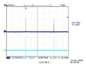
Figure 30: Short Circuit Protection at 12Vin, 5.0V out (40mS/div), Ch1: Vo, Ch2: Io, 50A/div
