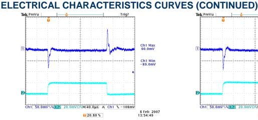
Figure 19: Transient Response at 12 Vin, 0.9V/40A out (40uS/div) Ch1: Vo, Ch2: Io, 10A/div
