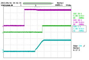
Figure 15: Turn on delay time at 12Vin, 1.8V/40A out (4mS/div) Ch2: PG, Ch3: Enable, Ch4: Vo
