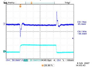
Figure 20: Transient Response at 12 Vin, 1.2 V/40A out (40uS/div) Ch1: Vo, Ch2: Io, 10A/div
