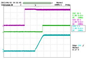
Figure 16: Turn on delay time at 12Vin, 2.5V/40A out (4mS/div) Ch2: PG, Ch3: Enable, Ch4: Vo
