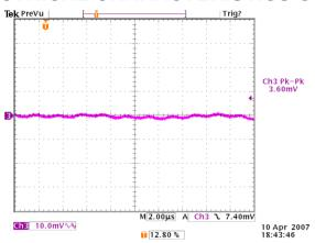
Figure 7: Output ripple & noise at 12 Vin, 0.9V/40A out (10mv/div, 2uS/div)
