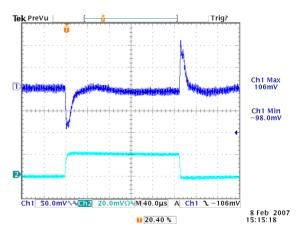
Figure 24: Transient Response at 12 Vin, 5.0V/40A out (40uS/div) Ch1: Vo, Ch2: Io, 10A/div
