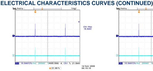
Figure 25: Short Circuit Protection at 12Vin, 0.9V out (40mS/div), Ch1: Vo, Ch2: Io, 50A/div
