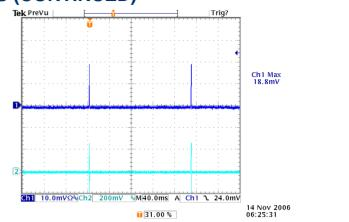
Figure 26: Short Circuit Protection at 12Vin, 1.2V out (40mS/div), Ch1: Vo, Ch2: Io, 50A/div
