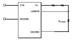
Figure 34: Circuit configuration for remote sense
