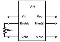
Figure 32: Enable input drive circuit example.
