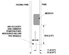
Note: Wind tunnel test setup figure dimensions are in millimeters and (Inches)
