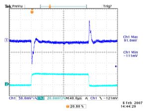
Figure 22: Transient Response at 12 Vin, 2.5V/40A out (40uS/div) Ch1: Vo, Ch2: Io, 10A/div
