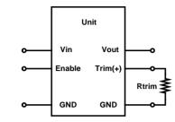
Figure 35: Trimming Output Voltage
