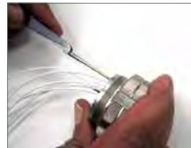
Removal of contacts with metal tool.
