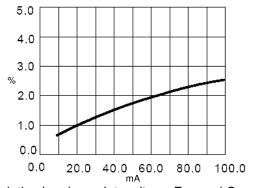
Relative Luminous Intensity vs Forward Current
