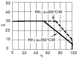
Maximum Forward DC Current vs Ambient Temperature
