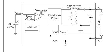
Figure 4 - RangeMAX Simplified Block Diagram
