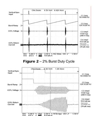
Figure 3 – 2% Burst Duty Cycle (Expanded Time Base)
