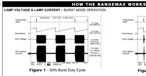
Rather than using the traditional dimming technique of varying lamp current magnitude to adjust light output, RangeMAX inverters use a fixed lamp current value with a duty cycle control method.
