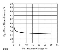
Fig. 6 - Diodes Capacitance vs. Reverse Voltage
