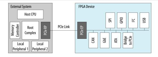
The Cyclone V PCIe hard IP operates independently from the core logic. This independent operation allows the PCIe link to wake up and complete link training in less than 100 ms while the Cyclone V device completes loading the programming file for the rest of the device.
