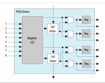
You can configure up to 25% of the ALMs in the Cyclone V devices as distributed memory using MLABs.
