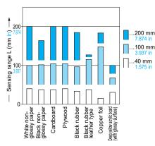
These bars indicate the sensing range with the respective objects when the distance adjuster is set to a sensing range of 200 mm 7.874 in, 100 mm 3.937 in and 40 mm 1.575 in long, respectively, with white non-glossy paper. Sensing object size: 35 × 60 mm 1.378 × 2.362 in.,
