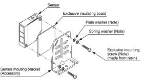
Note: Attached with the exclusive insulating board.
