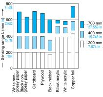
These bars indicate the sensing range with the respective objects when the distance adjuster is set to a sensing range of 700 mm 27.559 in, 400 mm 15.748 in and 200 mm 7.874 in long, respectively, with white non-glossy paper. (Sensing object size:  $35 \times 60$  mm 1.378 × 2.362 in.)
