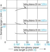
These curves show the characteristics with the maximum sensing range set to 200 mm 7.874 in. 100 mm 3.937 in and 40 mm 1.575 in, with white non-glossy paper (20 × 20 mm 0.787 × 0.787 in).
