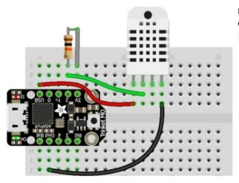
Here's an example using a Trinket M0 - you can use any CircuitPython board, just check that the Data pin is pulseio -capable.
