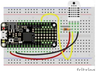
In this example we'll use a Feather M0 and DHT22 sensor connected to pin D6  $\,$
