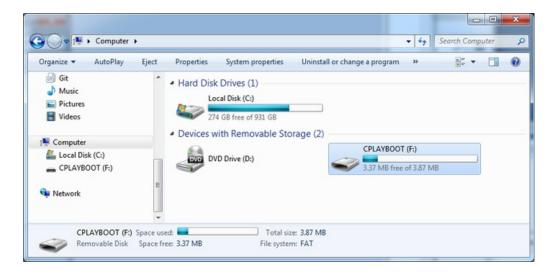
Once the bootloader is successfully connected you can open the drive and browse the virtual filesystem. This isn't the same filesystem as you use with CircuitPython or Arduino. It should have three files:
