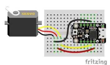
For example, to wire a servo to **Trinket**, connect the ground wire to **GND**, the power wire to **USB**, and the signal wire to **0**.
