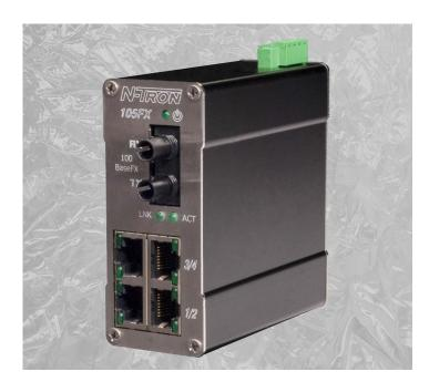
The 105FX supports up to 2,000 MAC addresses, enabling these products to support extremely sophisticated and complex network architectures.
